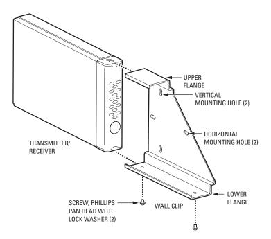
Figure 4. Mounting the FT8301A Transmitter/FR8301A Receiver Using the Wall Clip
